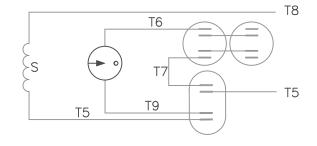
ROTATION JOIN & FACING L2 L1 **INSULATE** LEAD END P1 T4,T5 P2,T8 C.C.W. C.W. T4,T8 P2,T5 Р1
