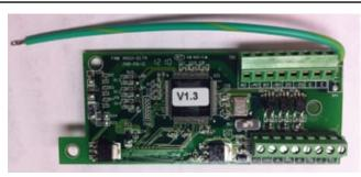
The A510 product has a standard RS485 port with RTU Modbus protocol. An optional card for Profibus Communications is available.
