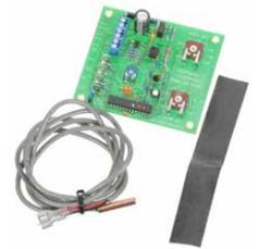
This control directly modulates ECM condenser fan motors via PWM signal in low ambient temperatures, varying the volume of air throughout the condenser, to regulate head pressure. Evergreen OM motor stock #'s 6301, 6303 and 6303R require PWM harness (stock 5K008) for compatibility with this control.
